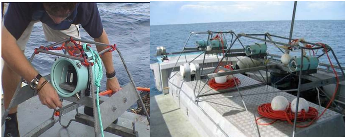
Figure 1: Cheap single (a, left) and stereo (b, right) systems using PVC pipe and acrylic housings in galvanised iron frames used in Australian shelf waters.
