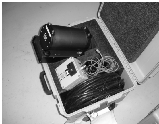
Figure 1: A standard unibody DIDSON transducer which weighs approximately 7kg and measures 171mm x 307 mm x 206 mm; b) A standard DIDSON accessory kit containing data cable, set-top box, Ethernet cables and the transducer. The operator additionally requires a laptop running DIDSON software to operate the unit.
